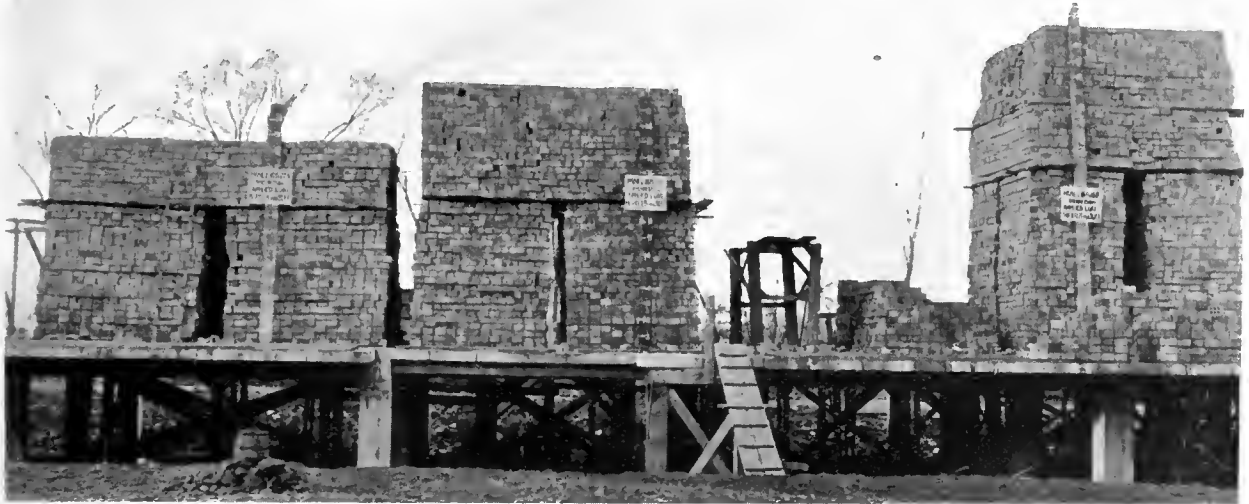
LOADING OF PANELS H, J AND K AT THE TIME OF THE NOVEMBER TEST Panels are lettered right to left
